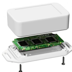
A 1.6 mm thick PCB can be clamped directly between the enclosure parts and optionally hot-caulked via two pins.
